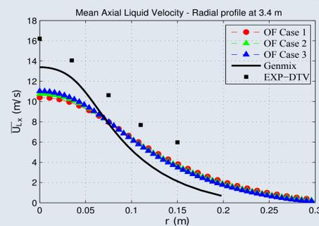
When comparing the liquid velocity radial profile 3.4 m from the nozzle in a case study, it is clear that modifications or new models are needed to better describe this type of flow.
