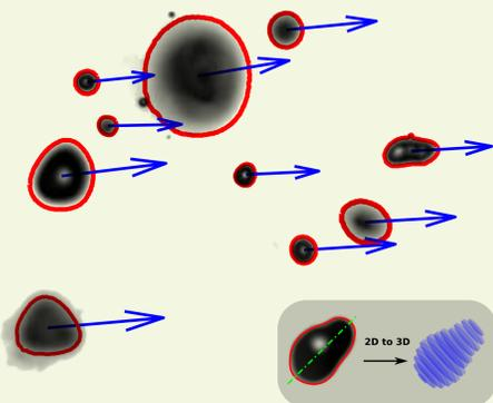
An In-house image processing algorithm was built to measure the liquid phase fields.
