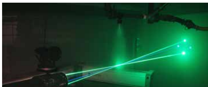
PDA laser for measuring the speed and size of spray drops
